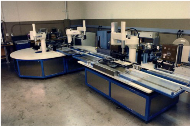
Figure 5 An assembly cell of AdeptOne SCARA robots for Xerox Corporation, 1986
