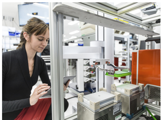
Figure 6 Ekaterina Mikhalev at Ginkgo Bioworks' in Boston, Massachusetts teaches the Precise Automation PF3400 SCARA, the world's first collaborative four-axis robot
